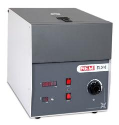
R - 23 & R 24 centrifuges are widely used in auxiliary laboratories in industry, Educational & Research institutions, Bio Technology, Medical Laboratories, Hospitals, Blood Banks, Pharmaceutical laboratories, Agriculture & Soil testing for determination of moisture equivalent of soil. It is also suitable for determination of settlement of paints, pastes, cosmetics and food products. Centrifuge rotors & carriers are also suitable for use with variety of Falcon & Vacutainer Tubes.
