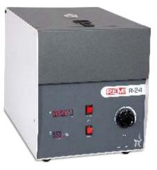
moisture equivalent of soil. It is also suitable for determination of settlement of paints, pastes, cosmetics and food products. Centrifuge rotors & carriers are also suitable for use with variety of Falcon & Vacutainer Tubes.
