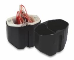
K 763- Set of 8 metal carriers suitable for rotor head K 761, having capacity to hold 2 blood bags in each carrier.
